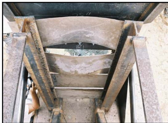
Figure 18. Witness Plates After Blast
