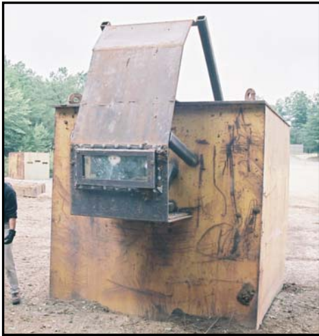
Figure 15. Shield After Blast
