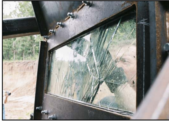
Figure 16. Window Interior After Blast
