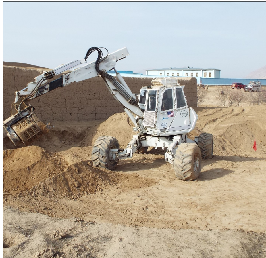
STORM with commercial sifting attachment reduces contaminated soil
