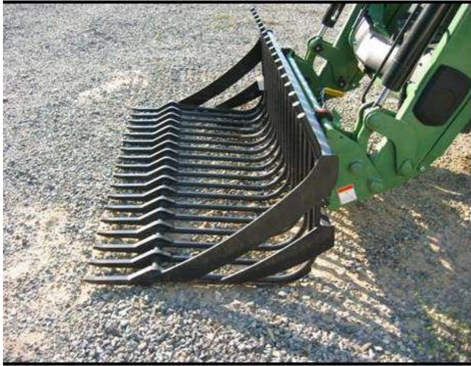
Figure 10: Quicke Rock Bucket (Stone Fork, Model 180)
