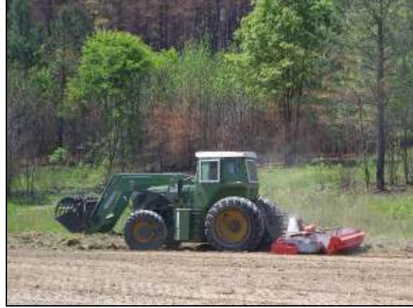
Figure 32: Power Harrow with Magnet Operations
