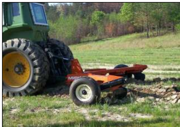
Figure 20: Operating Position, Miskin Parabolic Subsoiler
