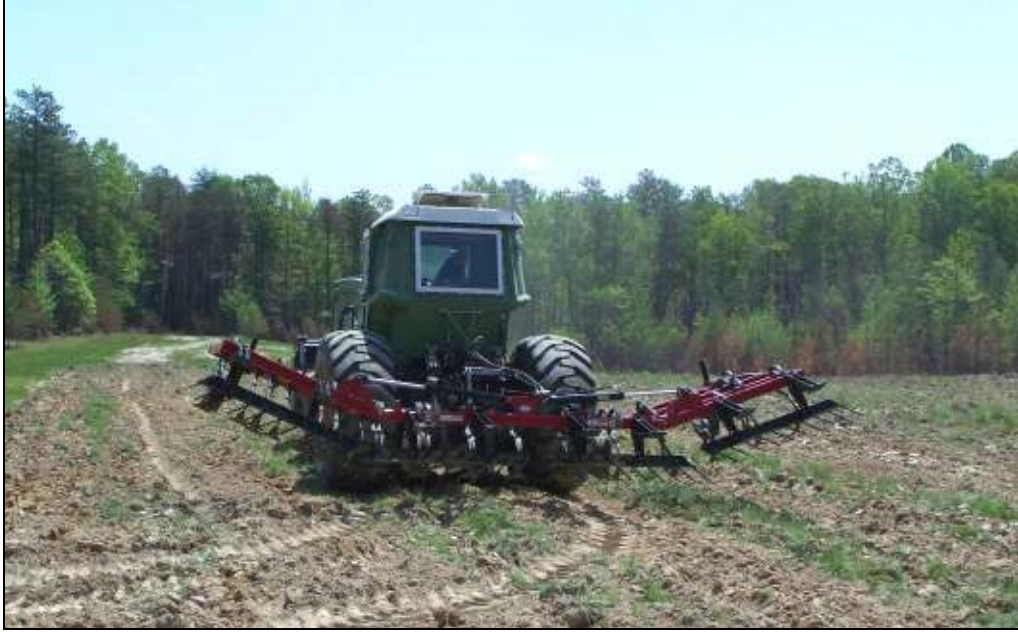
Figure 5: Unverferth Spring Cultivator Being Extended
