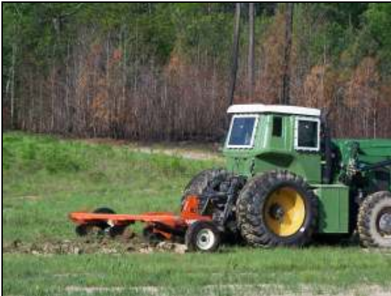
Figure 21: Miskin Subsoiler Operations
