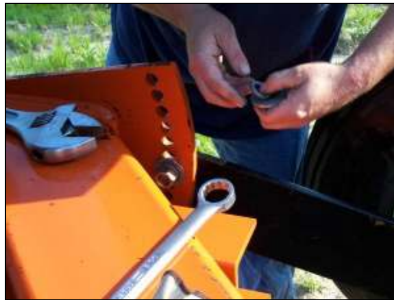
Figure 19: Height Adjustment, Miskin Subsoiler
