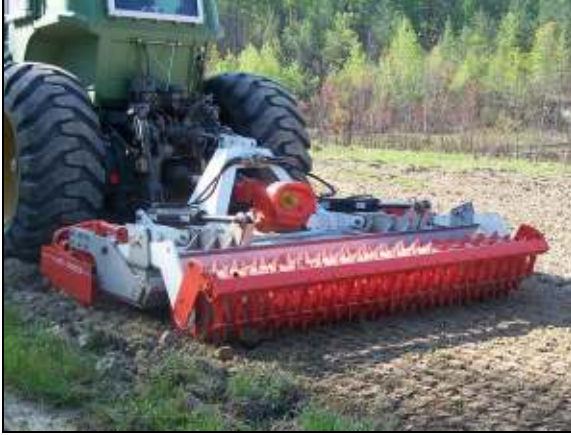
Figure 31: Power Harrow with Magnet Operations
