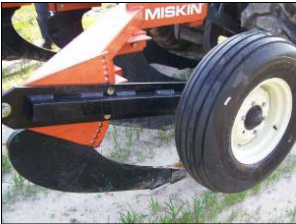
Figure 18: Height Adjustment, Miskin Subsoiler
