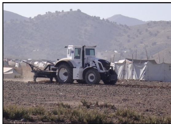
Left: RAPTOR II with its rotary mine comb attachment conducting anti-tank mine clearing operations with The HALO Trust in Afghanistan.
