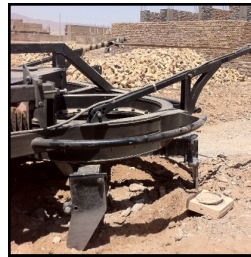
Above: RAPTOR 1's first AT mine. Right: Raptor with the rotary mine comb attachment near Jebrail, Herat, Afghanistan.
