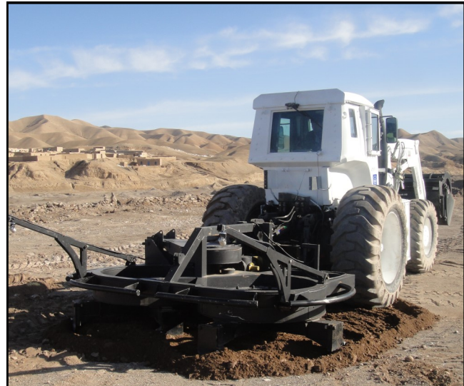
Above: RAPTOR 1's first AT mine. Right: Raptor with the rotary mine comb attachment near Jebrail, Herat, Afghanistan.
