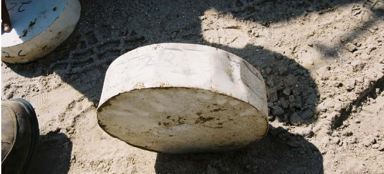
Figure 9. Example of Surrogate with Moderate Dent and Slight Case Buckling
