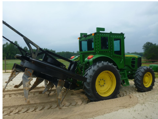
The RMC Lite project evaluated the use of a small frame tractor and a 3.1 meter RMC under light soil conditions
