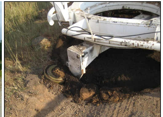
AT mine that the tines have engaged and nudged to the surface
