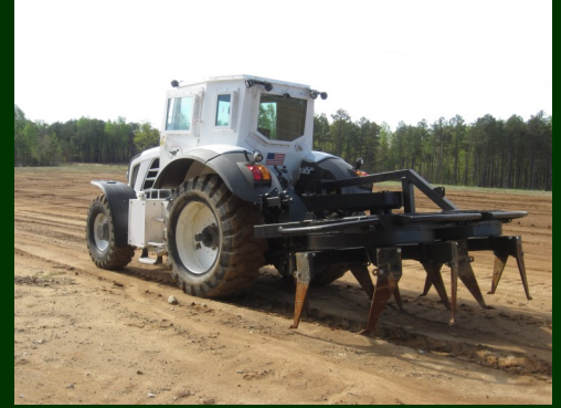
Intermeshing tines of the early RMC 4 tine design (left) and new six tine variant
