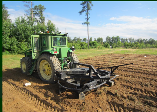
Improved 3.1 m wide RMC (left) and the 2.2 m system fitted to an ARMTRAC 75T
