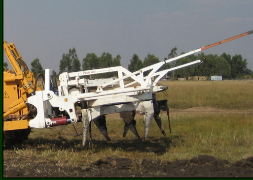
Intermeshing tines of the early RMC 4 tine design (left) and new six tine variant
