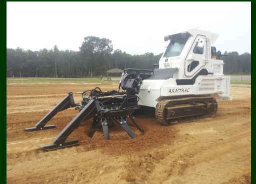
Improved 3.1 m wide RMC (left) and the 2.2 m system fitted to an ARMTRAC 75T
