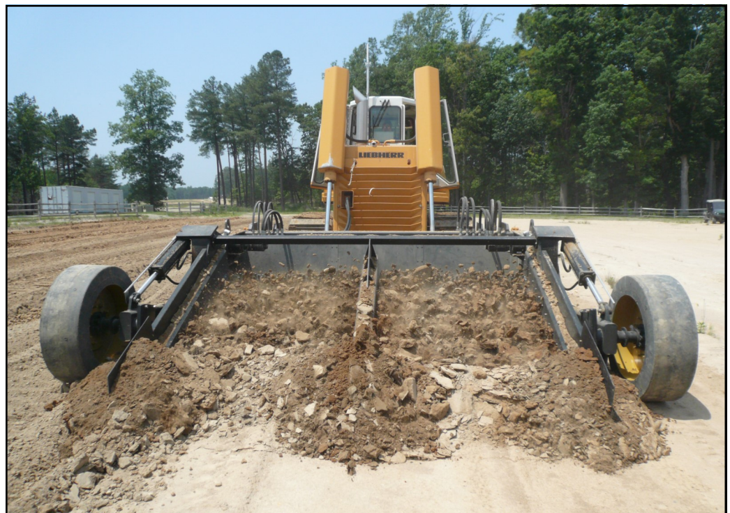
Soil travels up the sifting bed of the Mine Clearing Sifter during testing
