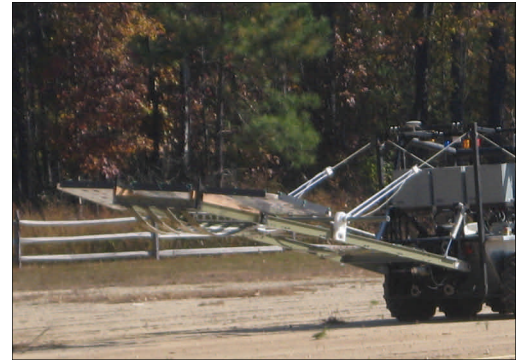
Ebinger UPEX 740 Deep Search Sensor Array
